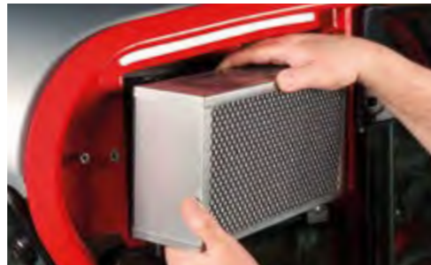
Large filters with quick and immediate access for ordinary maintenance.
