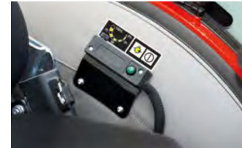
CONTINUOUS FLOW SETTING* Proportional electrical control for setting continuous oil flow up to 50 l/min.
