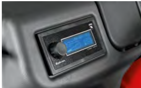
Air Control system, a liquid crystal digital display located on the driver's console that constantly records the pressurisation parameters within the cab showing the internal pressure values and the hours of operation of the Cat. 4 activated carbon filters.
