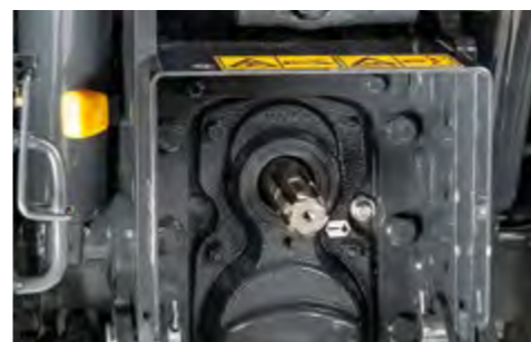
POWER TAKE-OFF PTO shaft with operating ranges 540/540E and standard.
