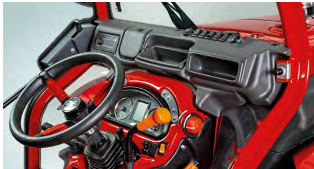
Protector 100 Cat. 4 CAB The cab enhances drive comfort providing extra object holders, a 12-volt plug for telephone recharging along with a pressure monitoring device that has a visual and acoustic alarm. Not to mention the possibility of hanging equipment displays fitted with digitalised control systems along the full length of the cab.
