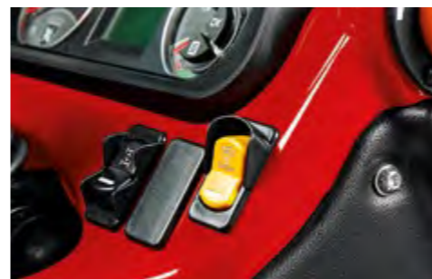
CONTROL TO KEEP PTO RUNNING This control keeps the PTO engaged and running even when the operator leaves the seat.
