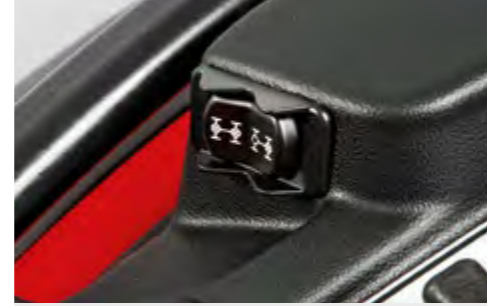
DIFFERENTIAL LOCKS CONTROL Engages, also under load, the differential lock either on both axles together or on the rear axle only.
