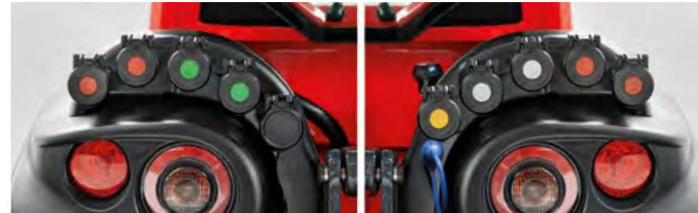
HYDRAULIC COUPLERS Optional hydraulic package* comprising 5 double-acting remotes, including 1 floating, 1 continuous delivery, 1 oil return and 1 drain return.
