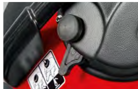
FLM (Fast Lift Management) Control for fast proportional raising and lowering of the linkage.
